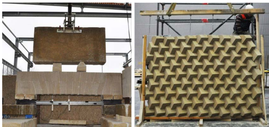
Figure 1. Prototypes in scale realized at the GAIA - Grands Ateliers de l'Isle d'Abeau in Villefontaine (Lyon) (coordination Prof. M. Brocato, ENSAPM): (on the left) model of the reinforced jack arch of the church of Saint-Sulpice in Paris, executed according to the design of Patte P. of 1769 (2011); (on the right) prototype of the façade panel composed of interlocking cubes (2013).
