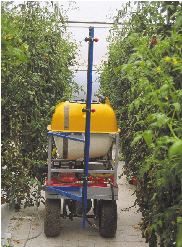
Figure 2. First prototype of the mobile platform used in the experiences reported in this paper. The platform carries on the spraying system shown in Figure 1b.
